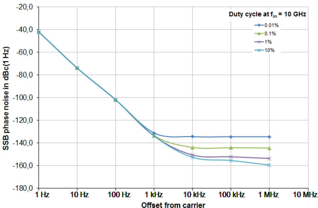
Typical phase noise sensitivity with R&S®FSWP-B60 option at  $f_{in} = 10$  GHz
